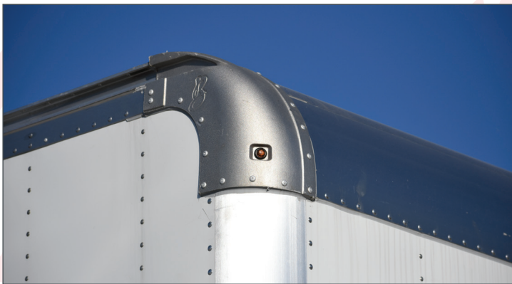
Unique aluminum corner cap design protects marker lights and ensures a strong impact resistant front end
